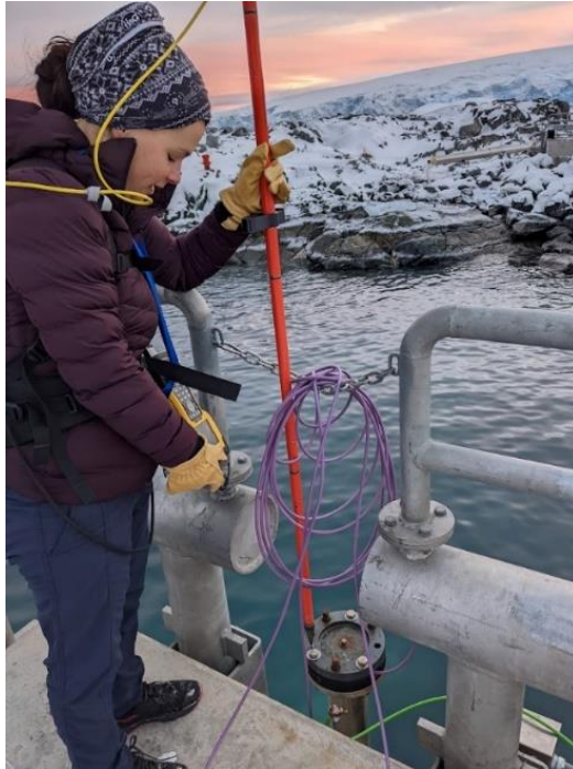
Figure 10. Performing a GPS survey of the newly reinstalled tide sensor – May 10, 2022.
